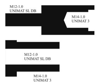
**Procedure:** Screw adapter on lathe spindle against a shoulder. Next screw lathe chuck on adapter against the shoulder on the adapter. Make sure that lathe turns towards you.
